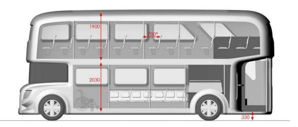
\* We have reduced the distance between seats to 700mm which is over the norm 2001/85/CE that says 650mm. This is done to reduce the length of the bus so a more compact bus can be achieved.
